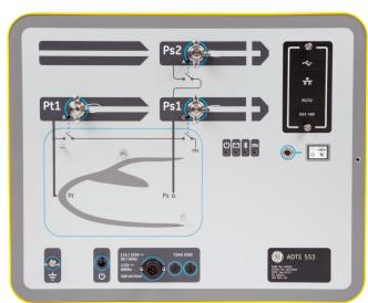
The ADTS553F air data test set is a portable three-channel flightline pitot static tester. It provides pitot static air data validation, leak testing, fault-finding and avionics instrumentation testing for any aircraft requiring angle of attack two off static-controlled channels, in addition to a pitot test channel. The ADTS553F can also be used as a standard two-channel flightline air data test set.
