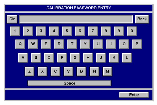
The Typewriter Keypad Entry screen is displayed when the SDX requires an alpha character input from the user. When the entry has been completed, select OK to continue.
