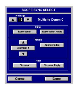
The Scope Sync screen is used to select the interrogation or reply that will be used to position the scope sync output. When a selection is made, the button text will turn yellow. To facilitate changing messages, the up and down arrows have been placed in the upper left corner of the screen. The available interrogation and reply options are a function of interrogation state (on/off) and message protocol.
